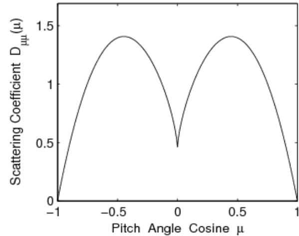
$$\lambda_{\parallel} = \frac{3v}{8} \int_{-1}^{+1} d\mu \frac{(1 - \mu^2)^2}{D_{\mu\mu}(\mu)}$$
