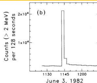
FIG. 1.—128 s accumulations of the counting rate of > 2 MeV gamma-rays at the *ISEE 3* spacecraft (Fig. 1a: 1980 June 21; Fig. 1b: 1982 June 3). The detector is a 1.4 kg CsI crystal enclosed in active anticoincidence shielding.
