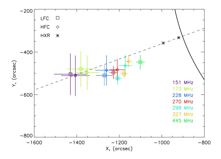
Relative positions of the LFC and HFC at several frequencies and of the HXR sources (average and scatter of the centroid positions) LFC always above HFC HFC component always a bit closer to the flare site
