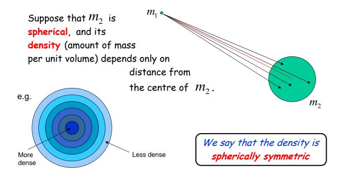
In this special case, the net gravitational force on  $m_1$  due to  $m_2$  is exactly the same as if all of the matter in  $m_2$  were concentrated in a point at the centre of  $m_2$ .
