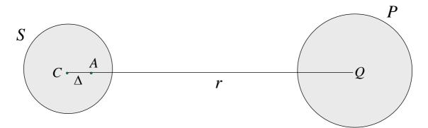
Tidal force between A and C due to the planet is equal to the difference in the gravitational force on A and C due to P
