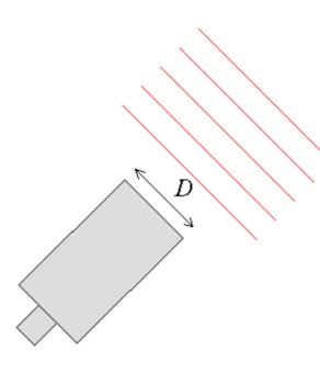
Light from a point source star arrives at a telescope aperture (of diameter D) as a series of plane waves
