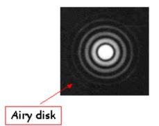
We can work out how the width of the Airy disk pattern depends on the size of the telescope aperture and the wavelength of the incident light.
