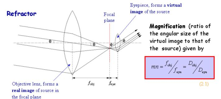
We can either view the virtual image through the eyepiece, or place a detector in the focal plane
