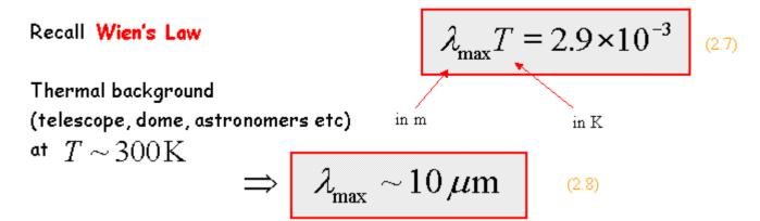
Cooling to about 100 K takes thermal peak outside of near infra-red range
