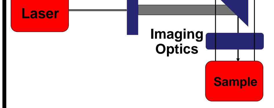
derives from macro scale PIV, where μΡΙV individual planes of the sample are illuminated via light sheet microscopy and then imaged. The light sheet thickness therefore defines the z-resolution. On the micro scale, illuminating individual planes is experimentally difficult and therefore the full volume is illuminated. The depth of correlation, related to (but not the same as) the focal depth of the microscope objective therefore defines the z resolution in  $\mu$ PIV.
