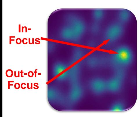
**DOC**: Because the full volume is illuminated, there will be a contribution to µPIV images from tracers outside the focal depth. Calculated vectors will influenced by these be effect particles; this İS quantified by the Depth of Correlation.
