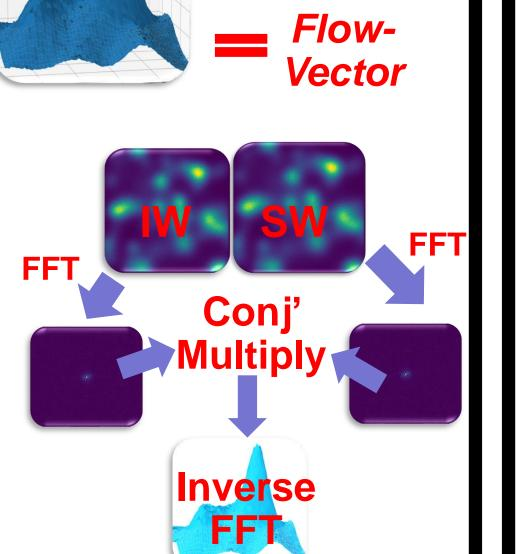
In Plane loss of pairs: Particles may not be present in both the IW and SW
