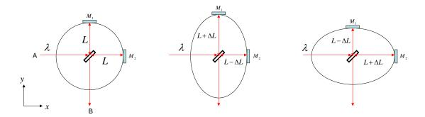
Figure 10: Cartoon illustration of the basic design features of a Michelson interferometer gravitational wave detector. See text for details.
