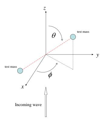
Figure 11: Cartoon illustration showing the relative orientation of a detector arm and the direction of propagation of a gravitational wave.
