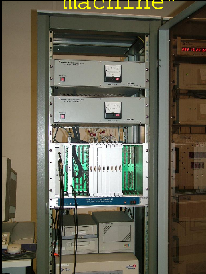
The Penn State Pulsar Machine II (PSPMII) a 2 x 64 x 3 MHz filterbank
